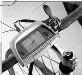
Handlebar mounted LCD data display and resistance control
